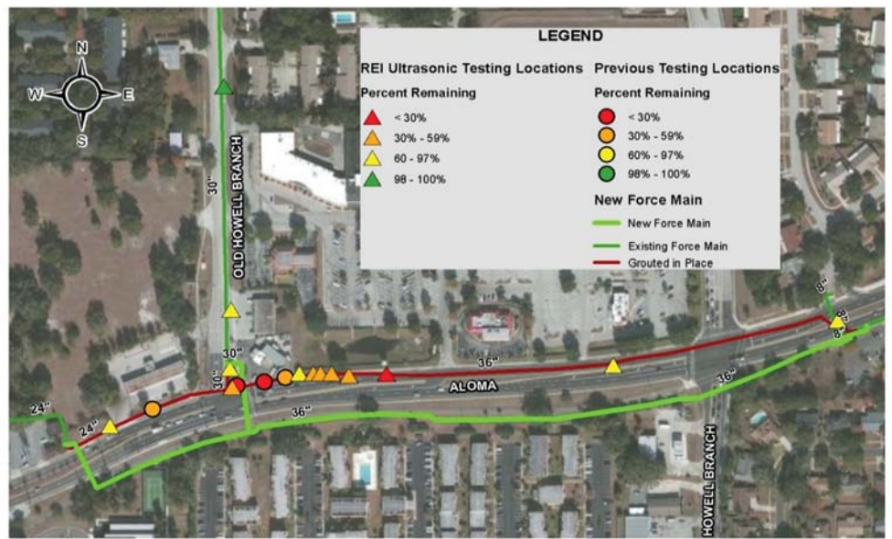
Figure 8. Replaced 36-in. Force Main on Aloma Avenue
